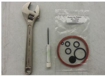
1. Tools Required •Wrench and small flat-head screwdriver •Pump-up repair kit •Brown/red Viton shown, blue EPDM available
